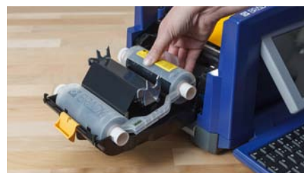
Drop and click print ribbons for 5-second ribbon supply changes
