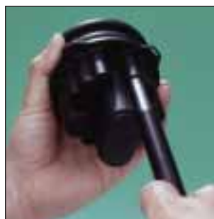
(1) Punch out base hole with port tool
